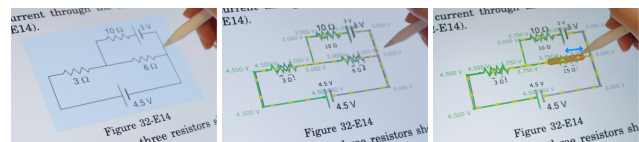
Figure 9: Augmented experiments for an electrical circuit diagram. 1) The user first selects a diagram. 2) The system then generates an overlaid simulation. 3) The user interacts with the simulation's values.
