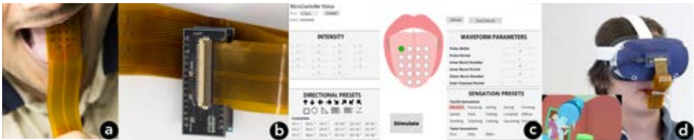
Figure 1: TactTongue is an oral interface that renders electro-tactile stimulations on the tongue. (a) It consists of an electrode array that can be placed on the tongue. (b) It connects to the Arduino Uno/Nano shield and comes in a compact form factor. (c) A design tool for prototyping diverse sensations and a few tastes on the tongue. (d) TactTongue can be deployed in diverse applications such as rendering the sensation of liquid flow when a VR character drinks water or lemonade.
