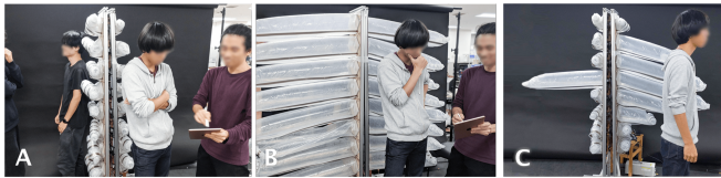
Figure 11: Adaptive space separation. The wall creates a temporary meeting space by separating the space, and changes shape to display an arrow.
