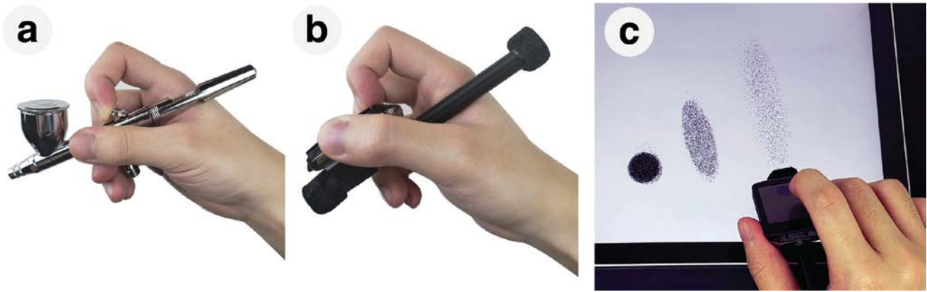
Figure 2. The Airbrush tool mimics the grip and control of a traditional airbrush. (a) A traditional airbrush is shown for comparison against (b) WatchPen acting as an airbrush; (c) shows examples of how the angle and the control of flow via the touch sensor can change the quality of the paint.
