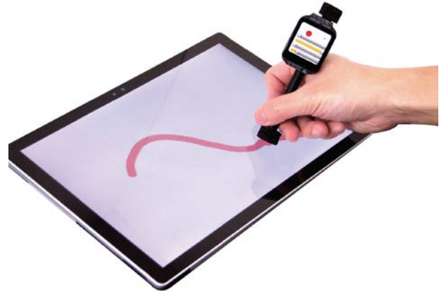
Figure 1. WatchPen is a prototype stylus which has been augmented with a smartwatch, thus providing rich cross-device capabilities to pen-based interaction.
