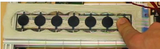
Figure 8: Slider made of 8 actuators in the same clamping area, and a capacitive slider underneath.
