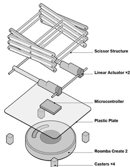
**FIGURE 8 |** The design of RoomShift, which integrates an expandable scissor structure with a Roomba robot.
