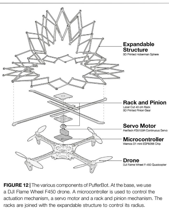
**FIGURE 12 |** The various components of PufferBot. At the base, we use a DJI Flame Wheel F450 drone. A microcontroller is used to control the actuation mechanism, a servo motor and a rack and pinion mechanism. The racks are joined with the expandable structure to control its radius.
