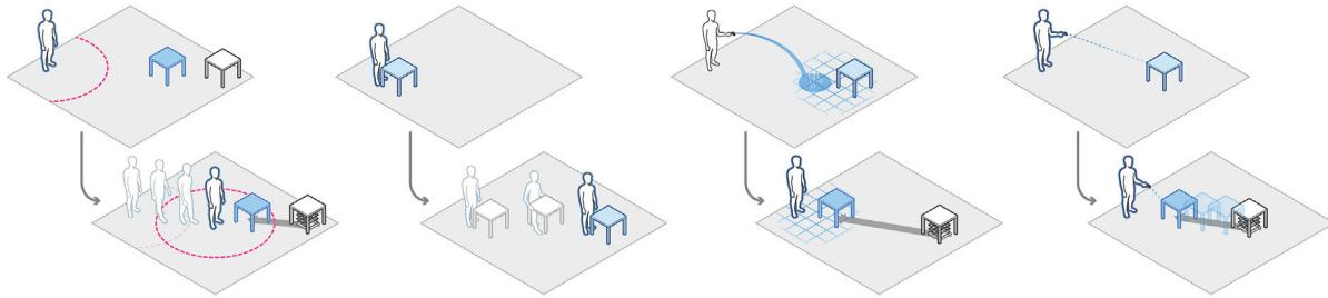
**FIGURE 9 |** RoomShift can provide encountered-type haptics for users in a variety of VR interactions, including when users walk to touch objects, physically move virtual objects, virtually teleport to new locations, and virtually move objects.
