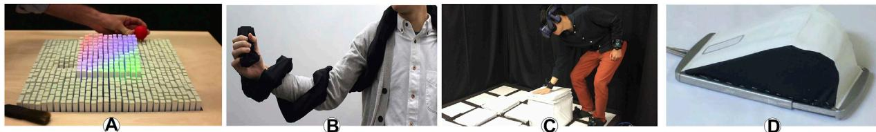
**FIGURE 2 |** Examples of various ways shape-changing interfaces researchers and designers have proposed to augment human-computer interaction: **(A)** dynamically actuated shape displays such as Materiable (Nakagaki et al., 2016b), **(B)** deformable, actuated linkages such as LineFORM (Nakagaki et al., 2015), **(C)** inflatable structures such as TilePoP (Teng et al., 2019), and **(D)** Inflatable Mouse: a volume-adjustable mouse with air-pressure-sensitive input (Kim et al., 2008).
