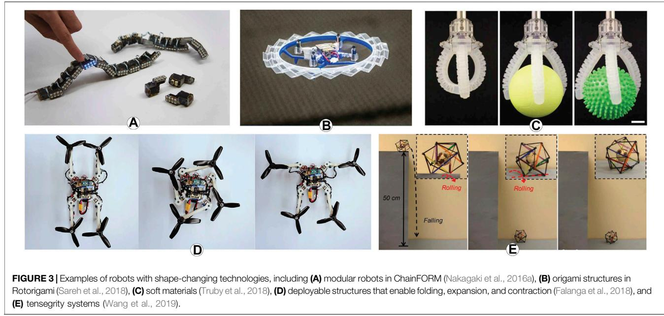
**FIGURE 3** | Examples of robots with shape-changing technologies, including (A) modular robots in ChainFORM (Nakagaki et al., 2016a), (B) origami structures in Rotorigami (Sareh et al., 2018), (C) soft materials (Truby et al., 2018), (D) deployable structures that enable folding, expansion, and contraction (Falanga et al., 2018), and (E) tensegrity systems (Wang et al., 2019).
