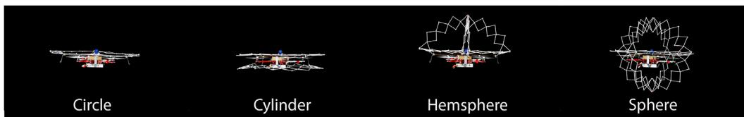
**FIGURE 11 |** We designed four varieties of expandable structures for PufferBot, each with trade-offs in the amount of protection it can provide, visual saliency for communication purposes, and weight.
